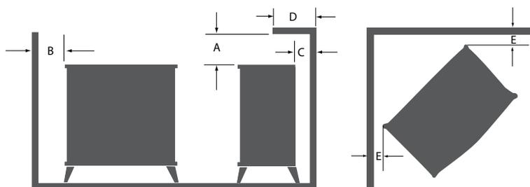
Vermont Castings direct vent gas stoves must be installed on rigid flooring. When the heater is installed directly on any combustible surface other than wood flooring, a metal or wood panel extending the full width and depth of the unit must be used as the hearth.
